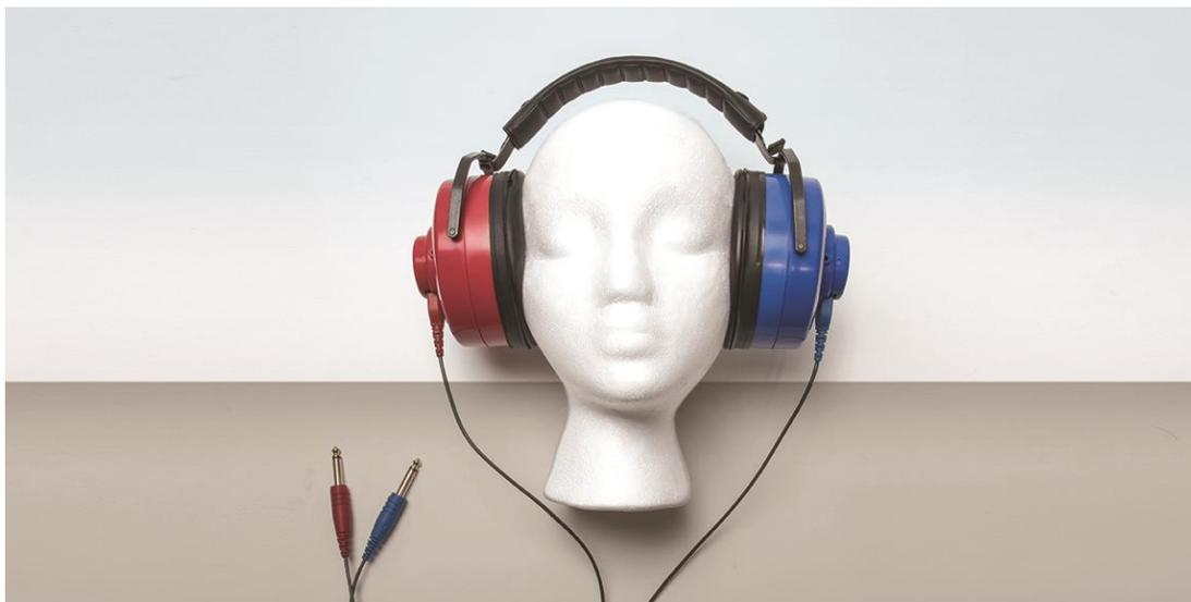
Custom-Designed Deep-Cavity Headset for the CCF-200 Fit Test
