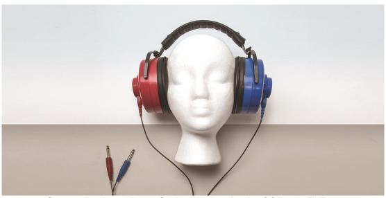
Custom-Designed Deep-Cavity Headset for the CCF-200 Fit Test
