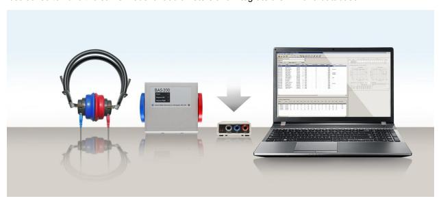
Benson Medical Instruments CCA-200 mini Computer-Controlled Audiometer and BAS-200 Bio-Acoustic Simulator
